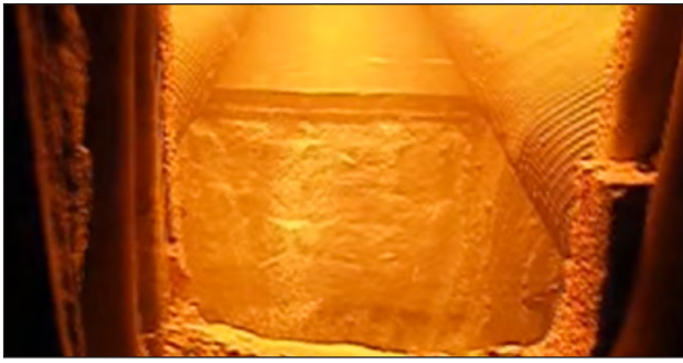
The crushed coal is blown into a furnace and burned at high temperatures
